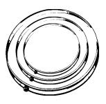
**DRAIN PANS AVAILABLE IN** 20" (508 mm) DIAMETER FOR WATER HEATERS HAVING A **DIAMETER 18" (457 mm) OR** LESS, 24" (610mm) DIAMETER FOR WATER HEATERS HAVING A DIAMETER 22" (559 mm) OR LESS AND AVAILABLE IN 28" (711 mm) DIAMETER FOR WATER HEATERS HAVING A DIAMETER 26" (660 mm) OR LESS.
